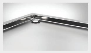
As an option, for harsher environments, we also offer a special anti-fingerprint finish: the 316 stainless steel surfaces first undergo a special micro shot-peening treatment and are then electropolished to create a bright, silk-smooth surface that doesn't compromise on cleanability or esthetics.
